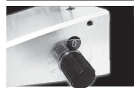
You mount your capillary tube on an oscillator. The vibrations cause the powder to drop down gently. Simply by turning one knob you can regulate the frequency of the oscillator to match the needs for each capillary tube/powder combination. This reduces the length of the procedure to an average of less than 1 to 2 minutes, depending on the powder.
